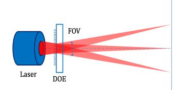
A DOE functions with a laser light source that emits a diffractive pattern. Each DOE pattern is characterized by a specific laser wavelength, focal length and transverse mode. Each laser wavelength will result in a different zero order intensity. The focal length is dependent on the DOE and the object distance which can be adjusted using a collimating lens (CL). The transverse mode will affect the dot shape.
